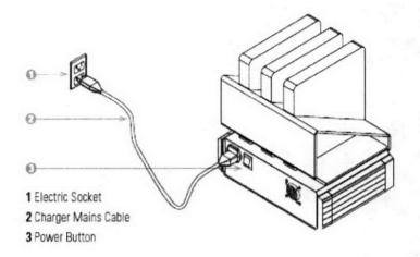
Back view of the battery charger and rack showing where to turn the charger on and off and where to connect the charger power cord
