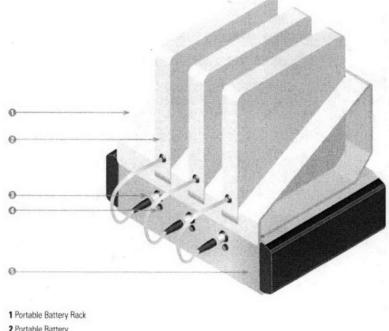
2 Portable Battery 3 Charger Socket 4 Charge Indicator 5 Charger
