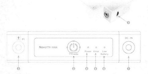
1 NovoTTF-100A power button 2 Connection cable socket (P1) 3 TTField therapy ON/OFF button 4 Power ON indicator light 5 Error indicator light 6 Low Battery indicator light 7 Battery connector socket
