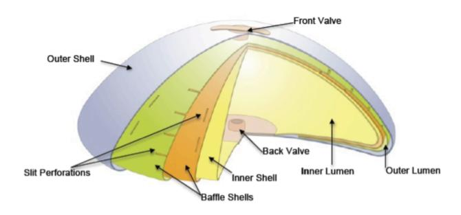
Cut-away of IDEAL IMPLANT (335 cc to 555 cc size) to show internal structure
