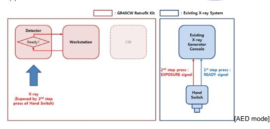
In conclusion, this retrofit kit does not either require a modification / alteration or control in the part of X-ray radiation control of the current X-ray system in anyway.
