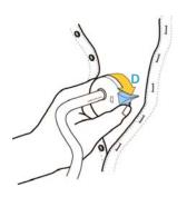
**Step 4:** Continue to push the Connector lever until it stops, then the Skin-Port valve is fully open.
