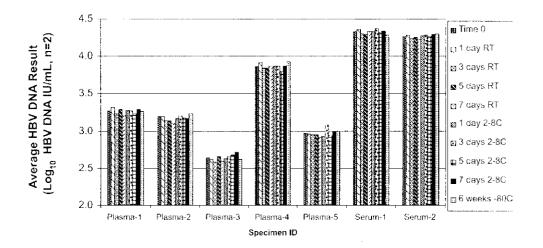
Serum and plasma specimens may be frozen and thawed up to five times without a loss of HBV DNA. The largest observed difference between the EDTA plasma conditions was not more than  $\pm 0.19 \log_{10}$  and the largest observed difference between the serum conditions was not more than  $\pm 0.10 \log_{10}$ . Figure below illustrates the HBV results after up to five freeze-thaw (F-T) cycles data from these freeze-thaw studies:
