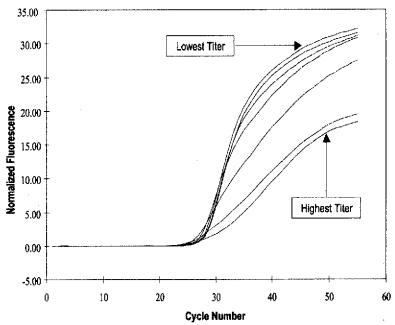
The fractional cycle number (Ct) is calculated where the fluorescence signal crosses the Assigned Fluorescence Level.
