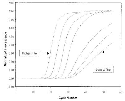
The amount of Quantitation Standard added to each specimen is constant for each reaction. The Ct value of the Quantitation Standard is similar regardless of the viral titer.
