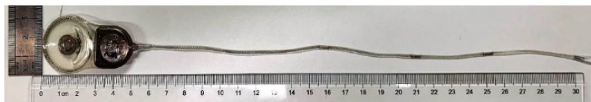
Figure 1: Minder Implant with telemetry unit and electrode lead.
