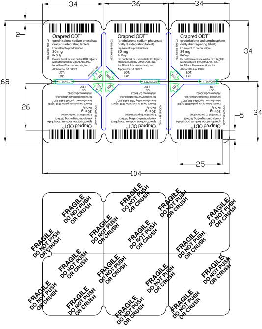
Bottom Foil is imprinted with the words: FRAGILE DO NOT PUSH OR CRUSH
