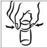
1. Open the solution bottle. Remove the safety cap by squeezing the tabs on the cap and twisting counterclockwise.
