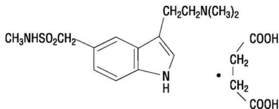
The empirical formula is C<sub>14</sub>H<sub>21</sub>N<sub>3</sub>O<sub>2</sub>S•C<sub>4</sub>H<sub>6</sub>O<sub>4</sub>, representing a molecular weight of 413.5. Sumatriptan succinate is a white to off-white powder that is readily soluble in water and in saline.
