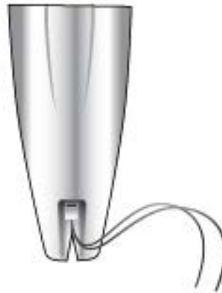
Figure 4: Securing the Threads in Cleft
