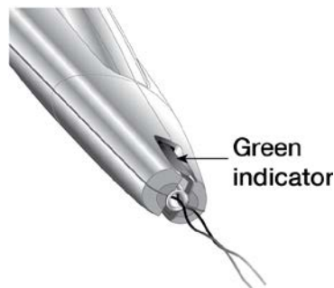
Figure 11: Green Indicator Visible and Threads Released from Cleft
