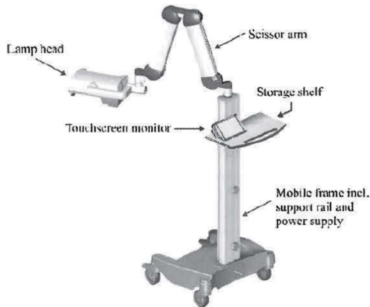
Figure 1- BF-RhodoLED® - key components
