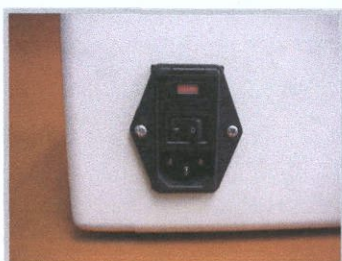
Image 1 - All LCU's come equipped with a 4-amp fuse to protect the unit from power surges. Always disconnect the power before accessing fuse.
