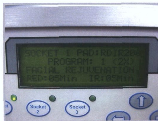
Image 4-The Socket Status Display pictured to the right shows that a main panel is plugged into socket one. The green light next to the socket one button indicates that socket one is ready.
