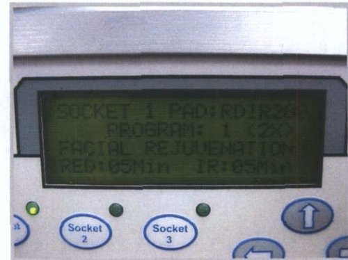
Image 4-The Socket Status Display pictured to the right shows that a main panel is plugged into socket one. The green light next to the socket one button indicates that socket one is ready.
