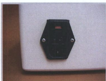
Image 1 - All LPCU's come equipped with a 4-amp fuse to protect the unit from surges. Always disconnect power before accessing fuse.
