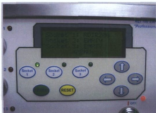
Image 3-The Main Control Display pictured to the left shows that a main panel is plugged into socket one and the green light next to the socket one button indicates that socket one is ready.
