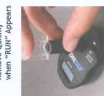
7b Press Shaker into Cartridge and Remove Quickly when "RUN" Appears
