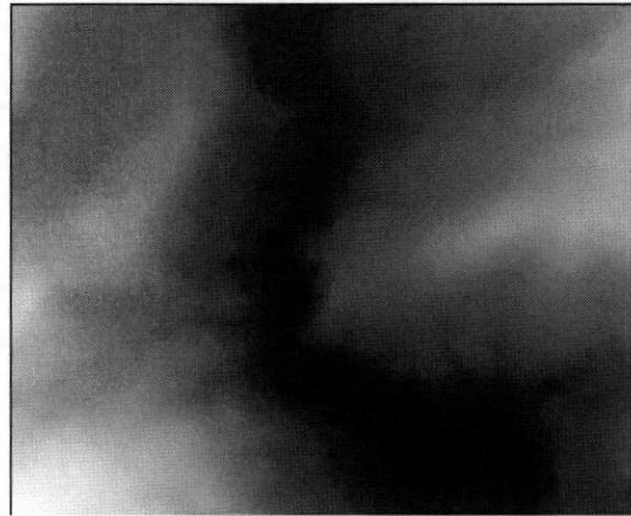
Fig. 16. DEM created by interpolating between isocontour lines in Figure 15.
