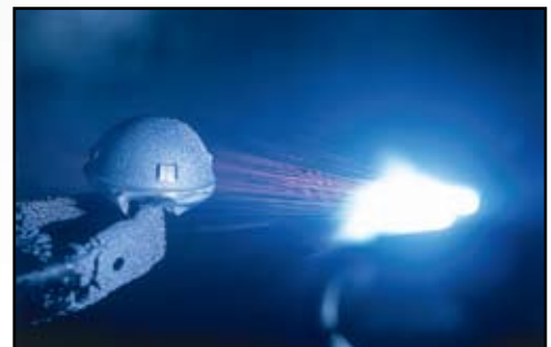
Titanium PPS® Porous Plasma Spray being applied through a heated plasma arc.
