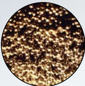
Fig. 5: Uniform sized beads results in uniform sized pores.
