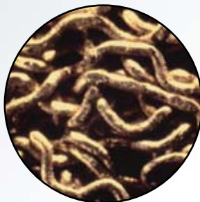
Fig. 6: Large pore structure of fiber mesh is the result of similar sized wires.
