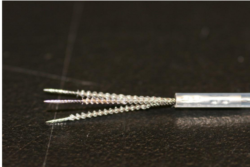
Figure 4: Triple Needle Tipped Brushes in advanced position
