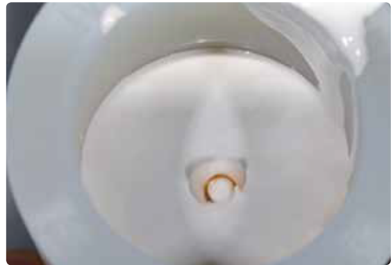
Pour the investment material slowly into the investment ring, so that the material can continuously fill the screw channel.
