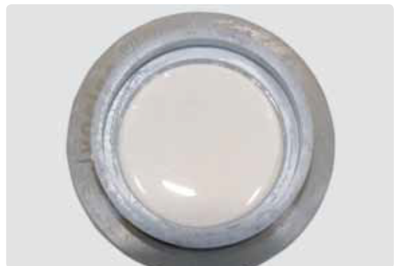
Continue to carefully fill the investment ring up to the marking and position the ring gauge with a hinged movement.
