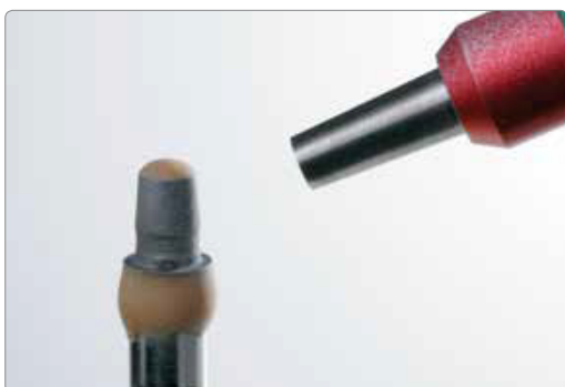
The bonding surface can be carefully blasted according to the instructions of the manufacturer.
