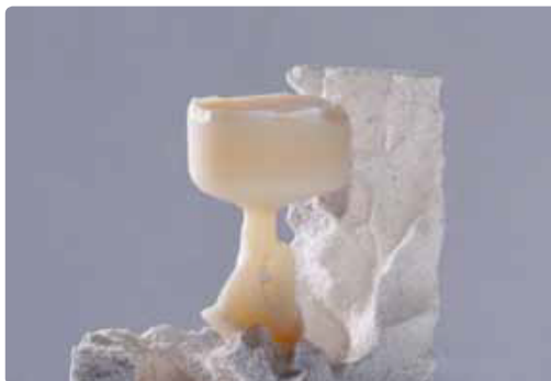
Fine divestment of the abutment is carried out with polishing beads at 2 bar (29 psi) pressure.
