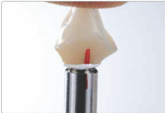
The ceramic structure is placed on the Ti base in such a way that the position markings are aligned. The components are joined using even and light pressure and the relative position of the components is checked (transition base/ceramic structure).
