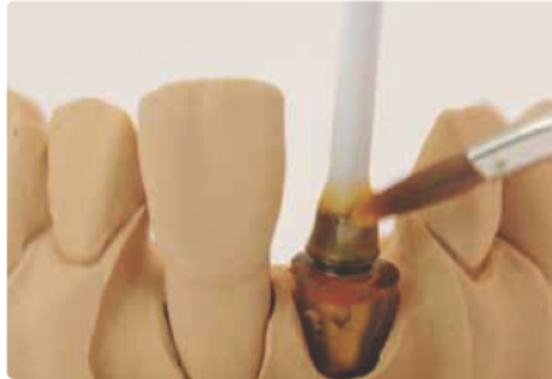
Apply the modelling resin to the Ti base in increments.
