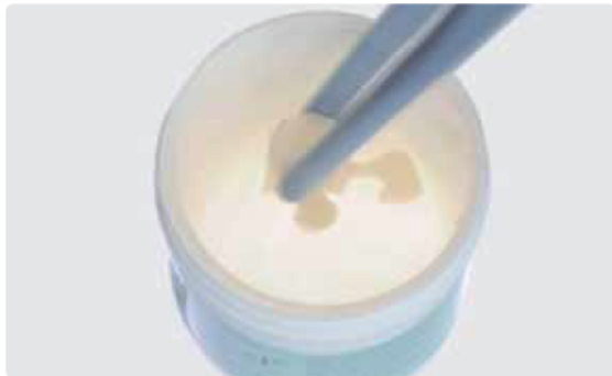
To remove the reaction layer, immerse the pressed objects in IPS e.max Press Invex ...
