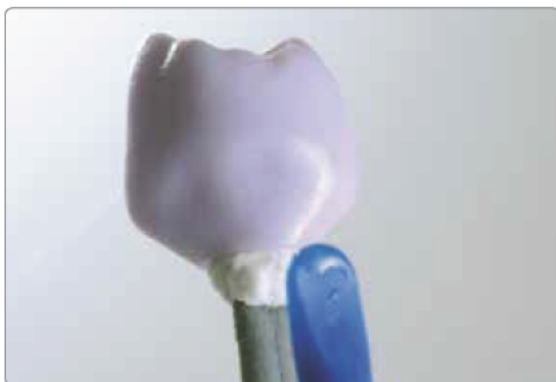
Displaced auxiliary firing paste is smoothed out with a plastic spatula from the margin towards the support pin so that the pin is secured in the paste.
