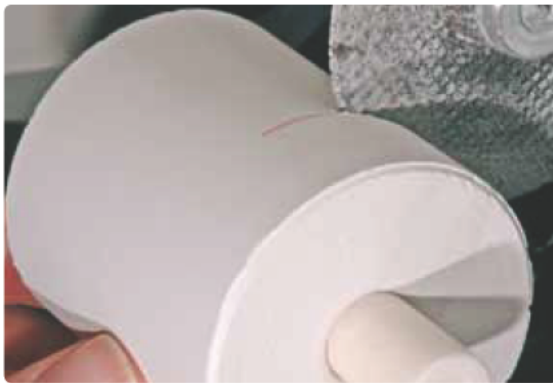
Separate the investment ring using a separating disc and break it at the predetermined breaking point.
