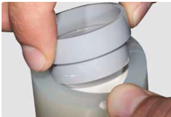
Continue to carefully fill the investment ring up to the marking and position the ring gauge with a hinged movement.
