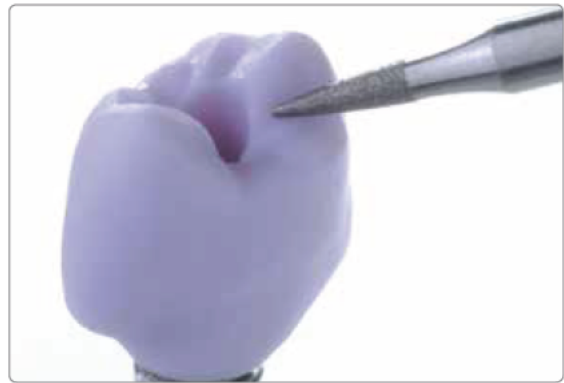
The surface of the ceramic structure is ground with a fine diamond to smooth out the surface structure created by the CAD/CAM procedure.
