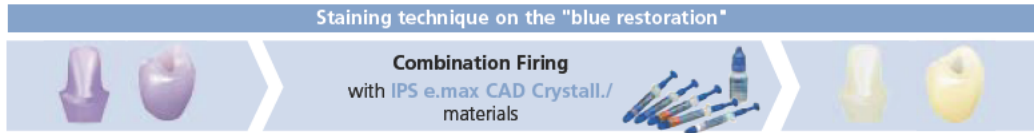
Characterization and glaze with IPS e.max CAD Crystall./ materials on the "blue" restoration, followed by Combination firing
