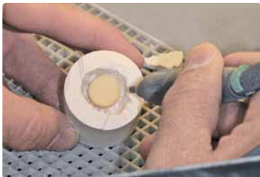
Rough divesting with polishing beads at 4 bar (58 psi) pressure until the object becomes visible.
