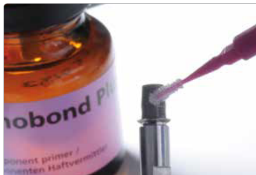
Monobond Plus is applied to the clean bonding surface and allowed to react for 60 s. After the reaction time, any remaining residue is dried with blown air that is free of water and oil.
