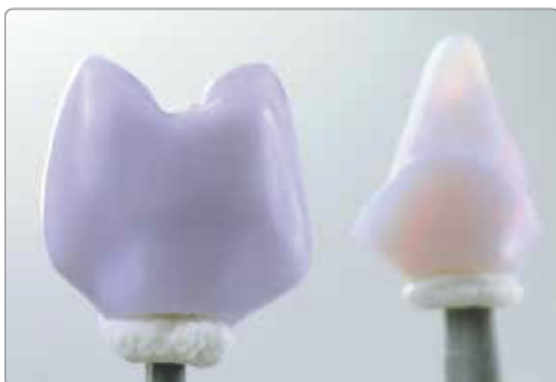
Important: – The IPS e.max CAD Crystallization Pin XS should be pressed only slightly into the IPS Object Fix Putty/Flow so that it does not touch the walls of the ceramic structure.
