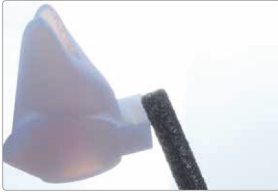
The attachment point to the block is smoothed out taking the shape of the emergence profile and the crown margin into account.
