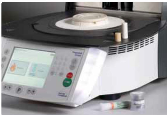
Provide a cold isolated IPS Alox Plunger and a cold IPS e.max Press ingot in the desired shade.
