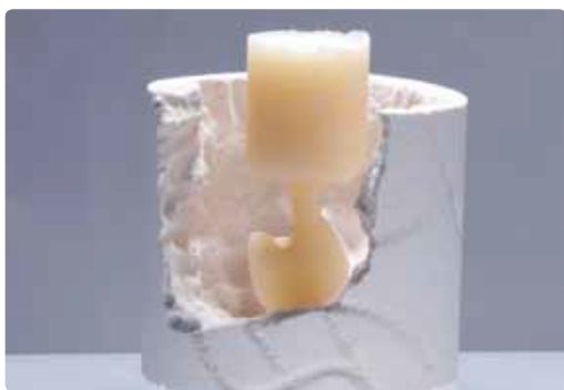
Fine divestment of the abutment crown is carried out with polishing beads at 2 bar (29 psi) pressure.
