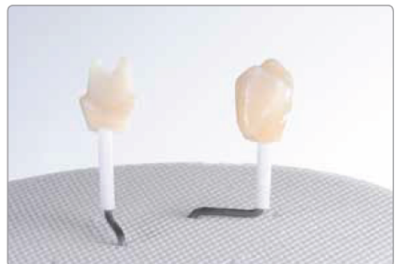
The Characterization/Glaze firing is conducted on a honey-comb firing tray with the corresponding parameters.
