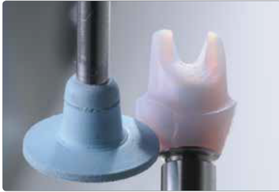
Pre-polishing by means of diamond rubber polishers
