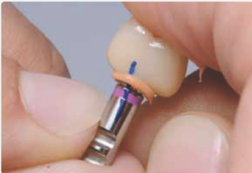
Insert the Ti base into the pressed object. In doing so, observe the relative position of the two components (rotation lock/markings). Hold the components in place for approx. 2:30 minutes until the Virtual Extra Light Body Fast Set material has set.
