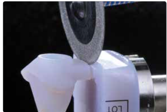
The attachment is cut from the basal using a diamond separating disc.
