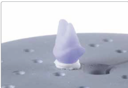
The interface of the ceramic structure is slightly overfilled with IPS Object Fix Putty or Flow. Then the ceramic structure is placed in the centre on the IPS e.max CAD Crystallization Tray.
