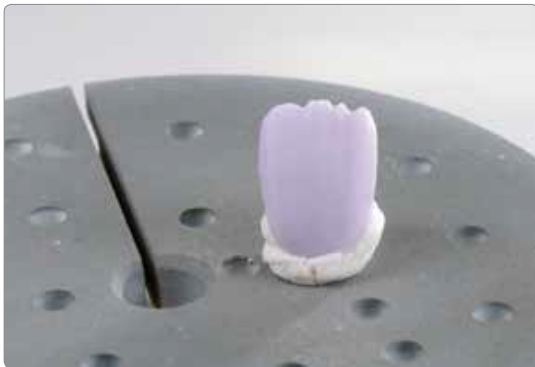
For crystallization, the partially reduced IPS e.max CAD restorations are placed directly on the IPS e.max CAD Crystallization Tray using IPS Object Fix Putty or Flow.
