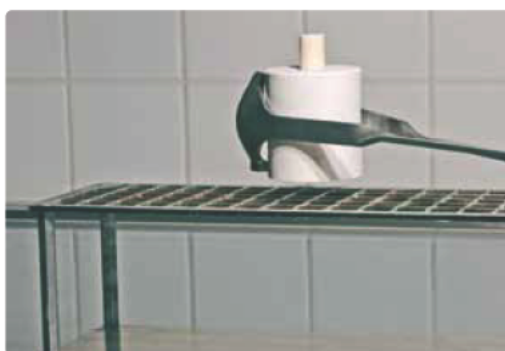
Once the press program is completed, place the hot investment ring on the cooling grid using the Investment Ring Tongs and allow it to cool to room temperature.
