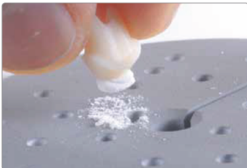
The ceramic structure is removed from the IPS e.max CAD Crystallization Tray.
