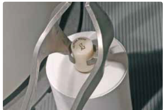
Place the cold IPS e.max Press ingot into the hot investment ring with the imprinted side facing up.
