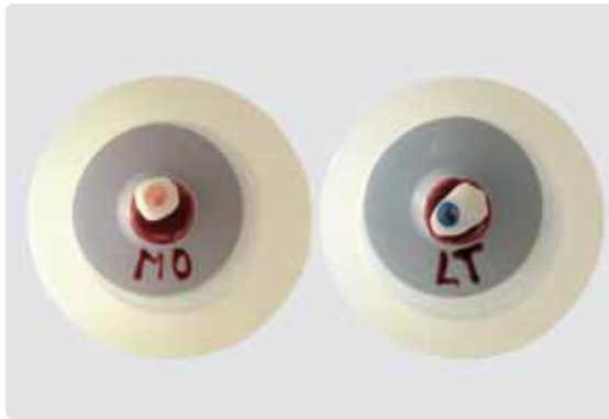
Correctly sprued abutment (left) and abutment crown (right). The screw channel is in a vertical position and parallel with the wall of the investment ring.
