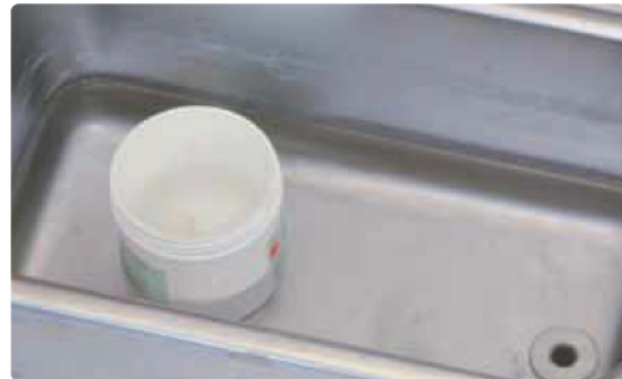
... and place in an ultrasonic cleaner for at least 10 and at most 30 minutes.
