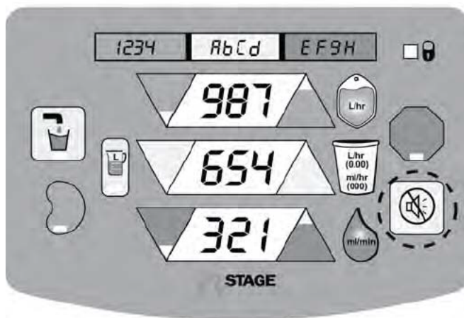
Figure 4-15: Second display test and MUTE key
