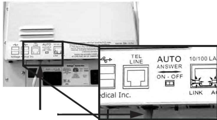
Figure 3-6: Telephone line connection
