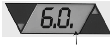
Figure 2-13: Pump ON indicator location
