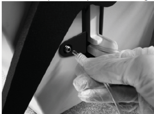
Figure 4-12: Connect the access pressure pod monitoring line
