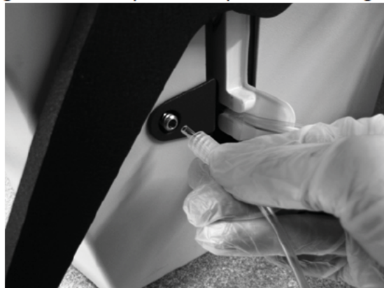
Figure 4-37: Attaching the access pressure pod monitoring line
