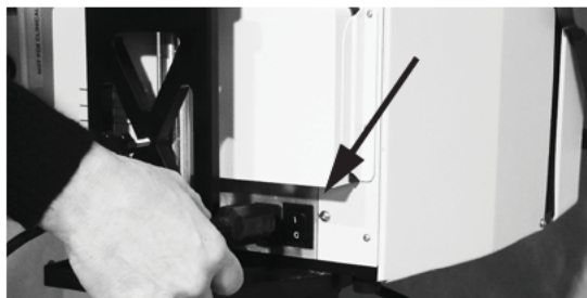
Figure 3-2: Power input for the cycler
