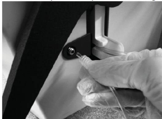
Figure 4-12: Connect the access pressure pod monitoring line
