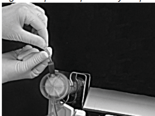
Figure 4-19: Loosening the cap of the post-dialyzer port
