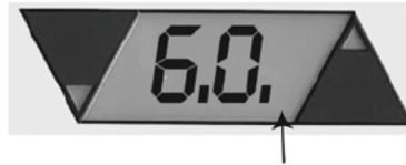
Figure 2-13: Pump ON indicator location
