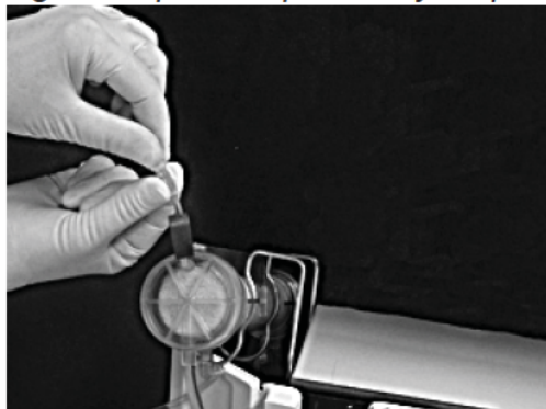
Figure 4-19: Loosening the cap of the post-dialyzer port
