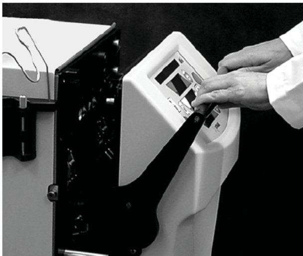
Figure 4-3: Open the cycler door
