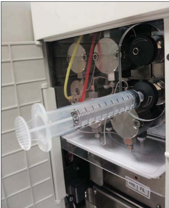
Figure 7-8: Syringe in Pump B Purge Valve
