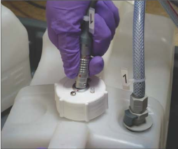
Figure 7-1: Disconnecting Level Sensor Cable from Waste Bottle
