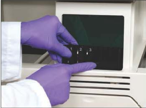
Figure 7-4: Removing Stat Rack
