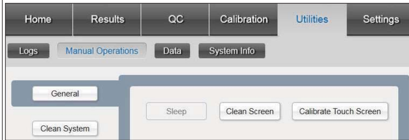
Figure 7-5: Utilities/Manual Operations Screen, Clean Screen Button
