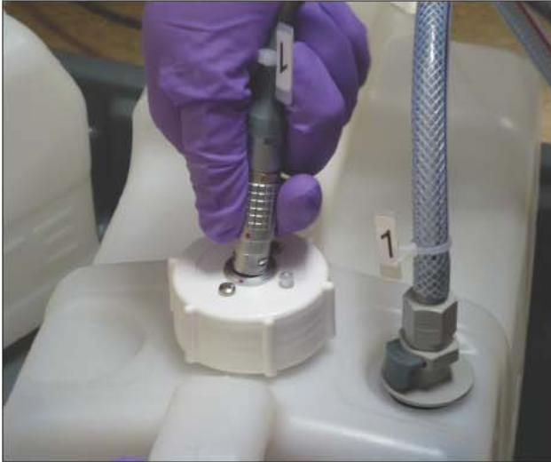
Figure 7-1: Disconnecting Level Sensor Cable from Waste Bottle
