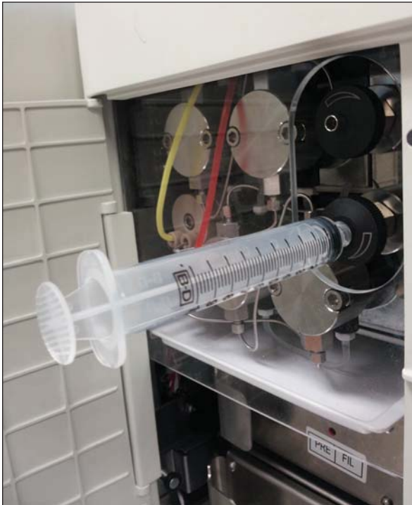
Figure 7-8: Syringe in Pump B Purge Valve
