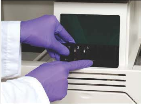
Figure 7-4: Removing Stat Rack
