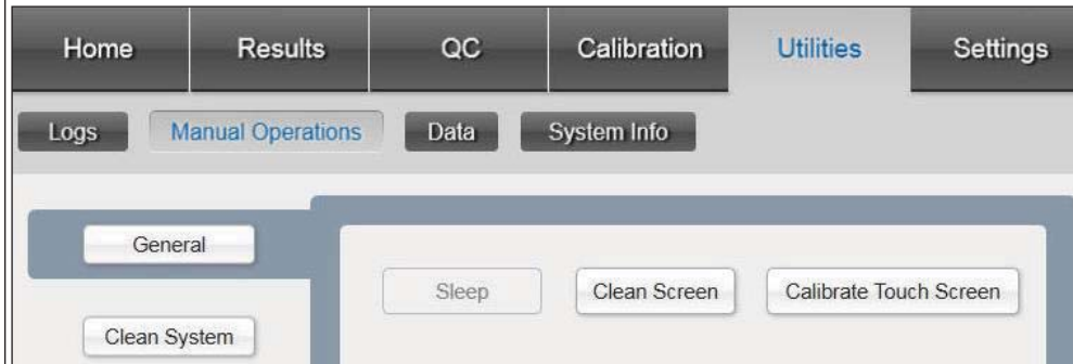
Figure 7-6: Utilities/Manual Operations Screen, Calibrate Touch Screen Button
