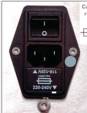
Figure 8-4: Fuse Inserted for 220-240 V
