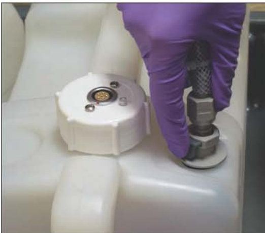
Figure 7-2: Disconnecting Waste Tubing from Waste Bottle
