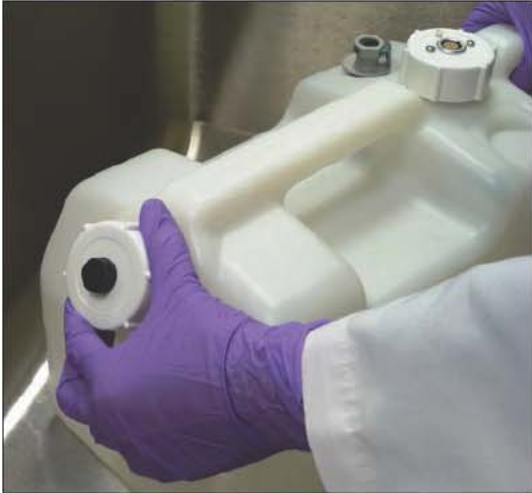
Figure 7-3: Unscrewing Waste Cap
