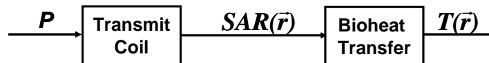
Figure 2. Flow-chart model of RF heating in MRI when there is no implant in the body. This figure is copied from reference [21].
