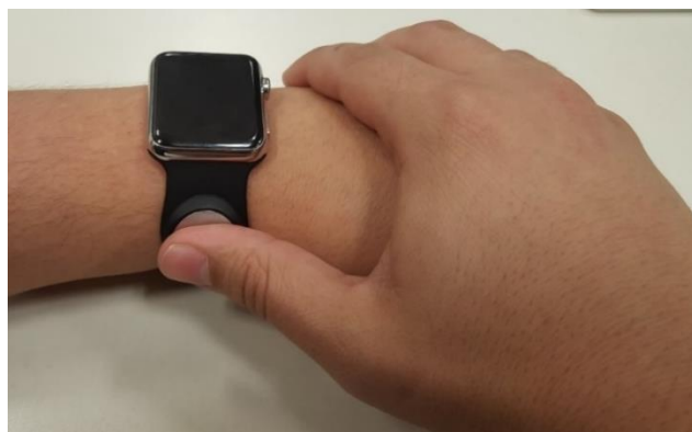
Figure 11.5. Recording an ECG with the Kardia Band System
