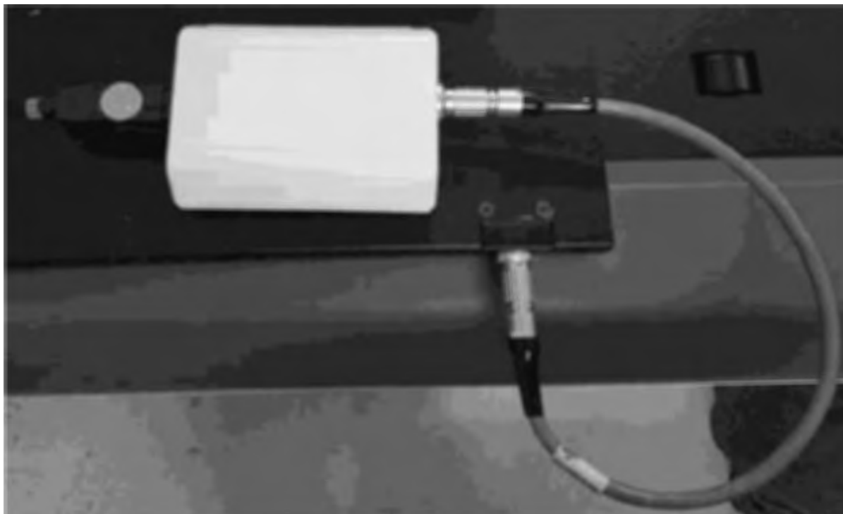
Light Box with Tracking Marker Cable and Couch Cable Connected
