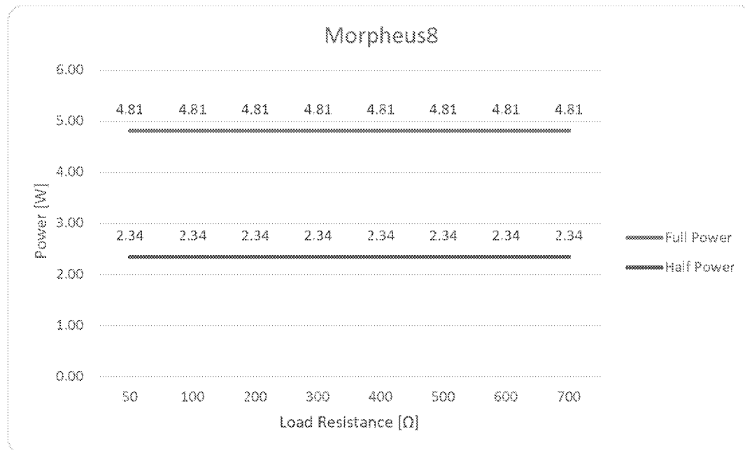
Figure 8-1: Morpheus Output Power versus Impedance
