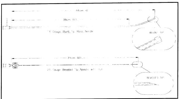
Fig. 5-3. 14 gauge curved Ross needle and 21 gauge needle with hub
