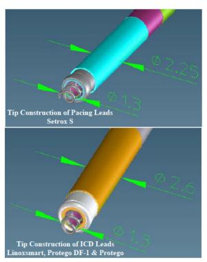
temperature profiles obtained from simulations, to show that the nearly 15 percent change in diameter has no substantial impact on the temperature rise near the helix. This is important since the ICD leads seem to be depositing higher amounts of power than the Setrox S 53 lead. The reviewers concern was expressed in Deficiency 1 of FDA's Major Deficiency Letter dated July 15, 2015:
