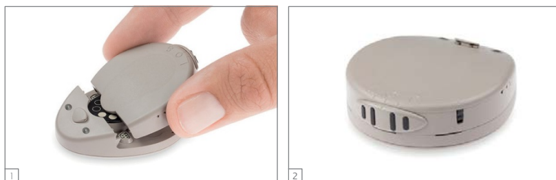
Fig. 17 Assembling the battery pack
