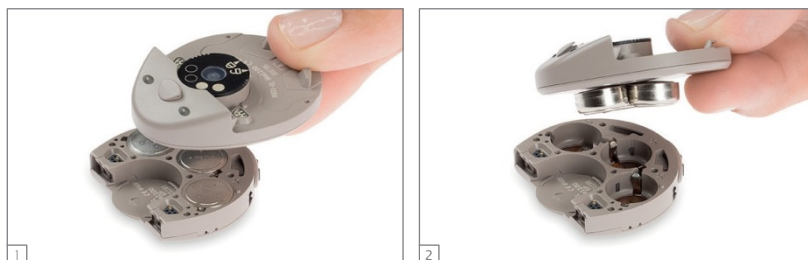
Fig. 16 Changing the batteries of your audio processor
