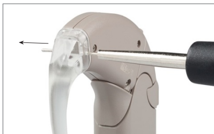
Fig. 21 How to remove the earhook pin
