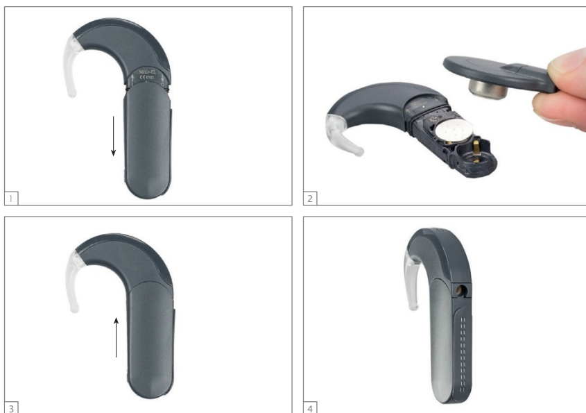
Fig. 35 Changing the batteries of your audio processor
