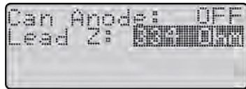
Figure 69. Lead Z field displays the system impedance.
