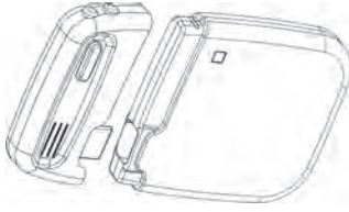
Figure 9. Connecting the EPG header to the EPG
