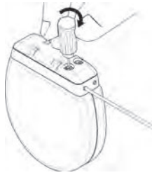
Figure 5. Tighten the setscrew clockwise
