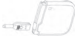
Figure 8. Inserting the connector into the EPG stimulator port
