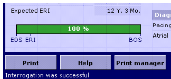
Figure 2: Battery Indicators on the Programmer Screen
