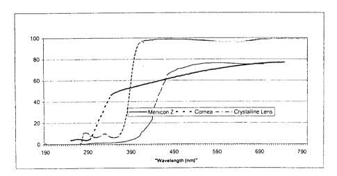
Menicon  $Z^{\text{TM}}$  (tisilfocon A) Contact Lens - Spectral transmittance curve for Menicon  $Z^{\text{TM}}$  (tisilfocon A) Contact Lens - D & C Green No. 6 and UV absorbing agent (sample thickness Menicon  $Z^{\text{TM}}$  (tisilfocon A) lens polymer plate = 0.08mm, representing the thinnest marketed version of the lens).
