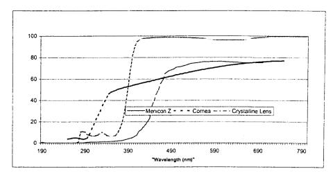
MENICON  $Z^{TM}$  (tisilfocon A) Contact Lens - Spectral transmittance curve for Menicon  $Z^{TM}$  (tisilfocon A) Contact Lens - D & C Green No. 6 and UV absorbing agent (sample thickness Menicon  $Z^{TM}$  (tisilfocon A) lens polymer plate = 0.08mm, representing the thinnest marketed version of the lens).
