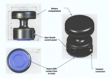
PRINCIPLES OF OPERATION: Active Signal's stethoscope combats noise intrusion through use of two modes of operation depending on the intensity of background noise:
