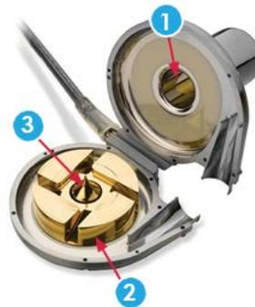
The pump displaces 50mL of blood, weighs 160g, and is capable of pumping up to 10 liters per minute (L/min) of blood. It is designed to be implanted entirely in the pericardial space, obviating the need for an abdominal pocket.
