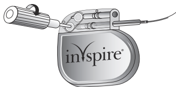
Figure 17. Tighten the lower setscrew
