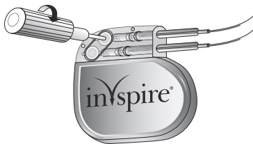
Figure 19. Tighten the upper setscrew
