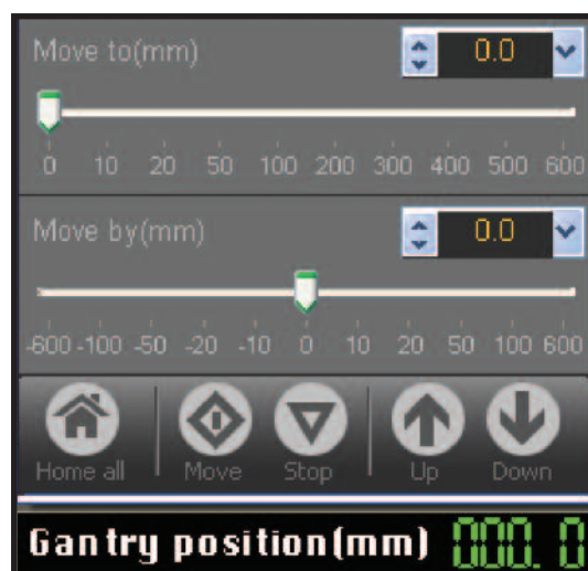
Figure 13.5.1-2: Adjusting the gantry's vertical position
