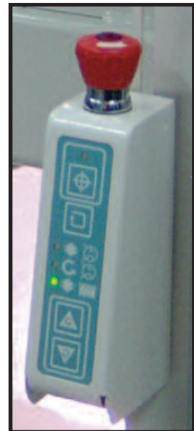
Figure 13.6.1-2: Scanner control panel
