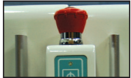
Figure 6.1.1-1: Emergency Stop button
