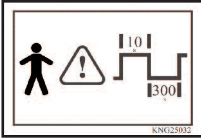
Figure 5.2-6: Duty cycle label
