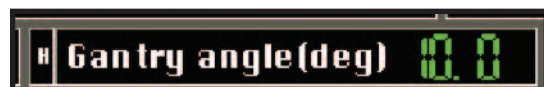
Figure 13.5.1.1-1: Home light is not lit; gantry is not at its angular home position
