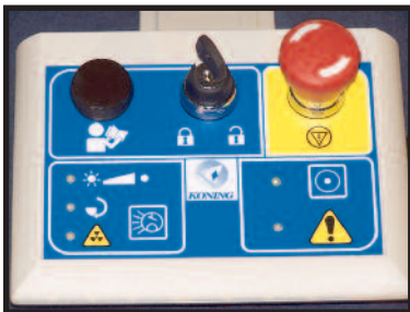
Figure 16.2-2: Emergency stop button found on the control panel at the Operator's Console
