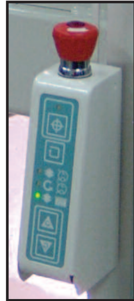
Figure 13.5.1-3: Scanner control panel
