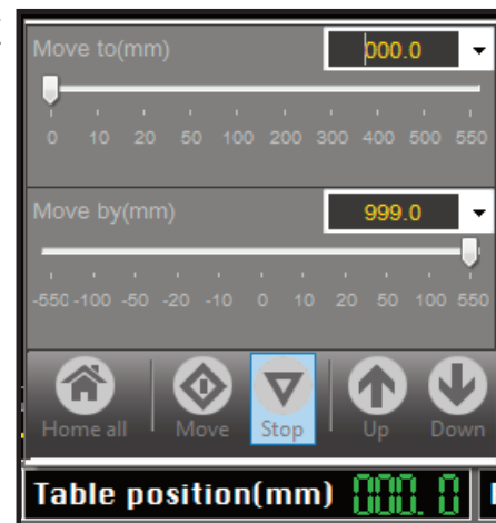
Figure 16.2-5: Stopping a moving part
