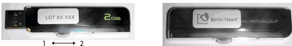
Fig. 16-6 Left: USB stick with extended plug (operating position); Right: USB-stick with retracted plug (position to transport and store the stick)
