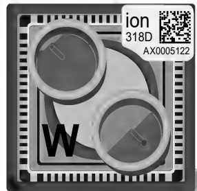
Chip marked for water wash/initialization:
