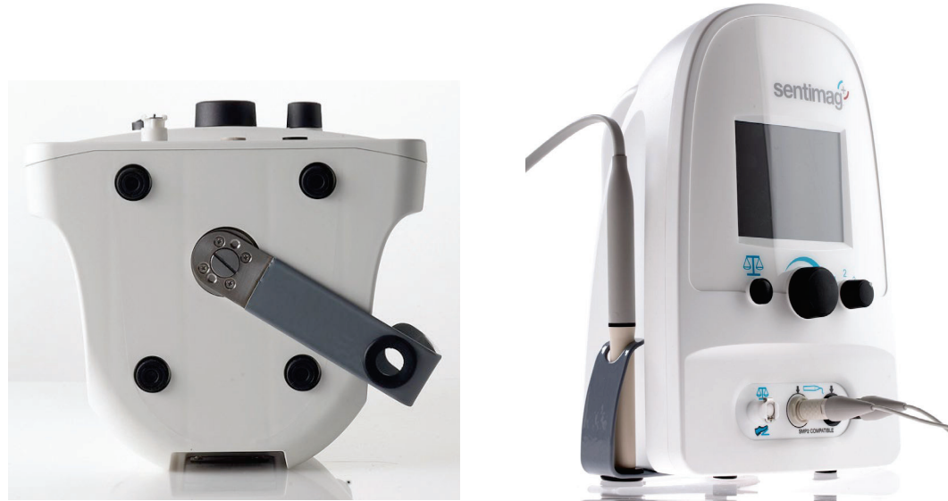
Figure 6: (a) connection of the probe holder, and (b) use of the probe holder.
