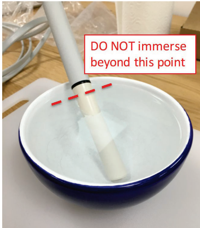
Figure 11: Immersion of probe head in disinfection solution
