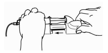
Figure 6.21 Installing the Syringe to the Infusion Pump
