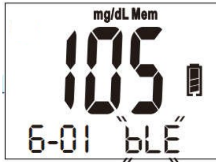
Fig. 4 “bLE” and test time on meter’s display flash alternately during data transmission
