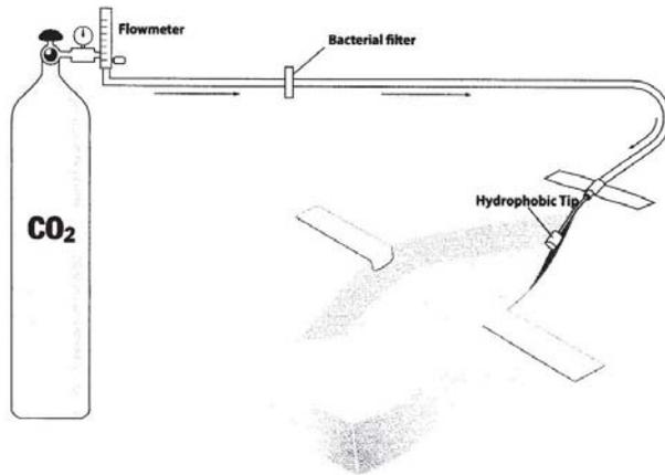
Figure 4.1: How the TEMED Gas Diffuser might be used. The device is connected to regulated carbon dioxide gas source, the gas flows through the tubing, through the bacterial filter, through a further length of malleable tubing and then out through the hydrophobic tip.
