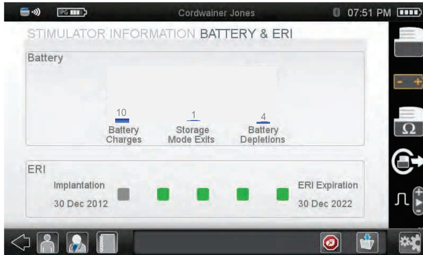
Figure 30. Battery & ERI screen
