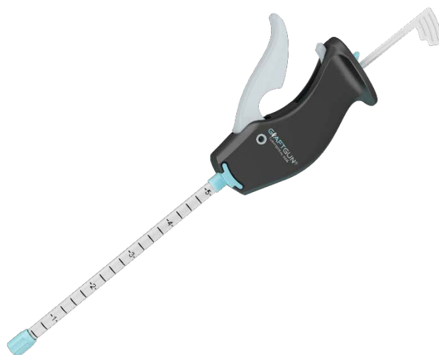
Figure 1 Fully assembled Graft Gun dispensing unit. The unit graft tube is to the left and the base of the plunger is shown to the right. Upon squeezing the trigger mechanism on the handle, the plunger is advanced down the length of the graft tube to express the graft material from the graft tube tip into the intended graft site. The graft tube is 7.17 inches in length with a diameter of .350 inches. The component is made up of medical grade polypropylene.
