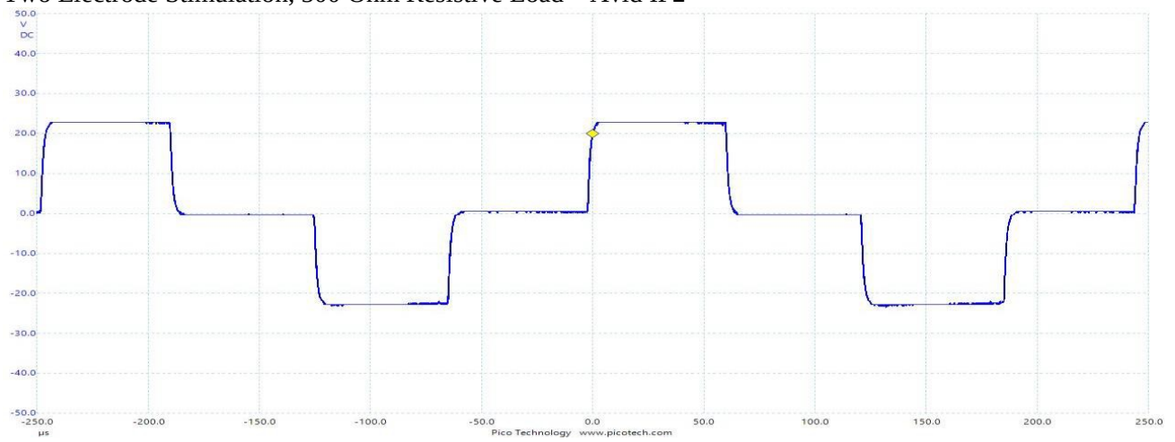
Two Electrode Stimulation, 500 Ohm Resistive Load – Avid IF2
