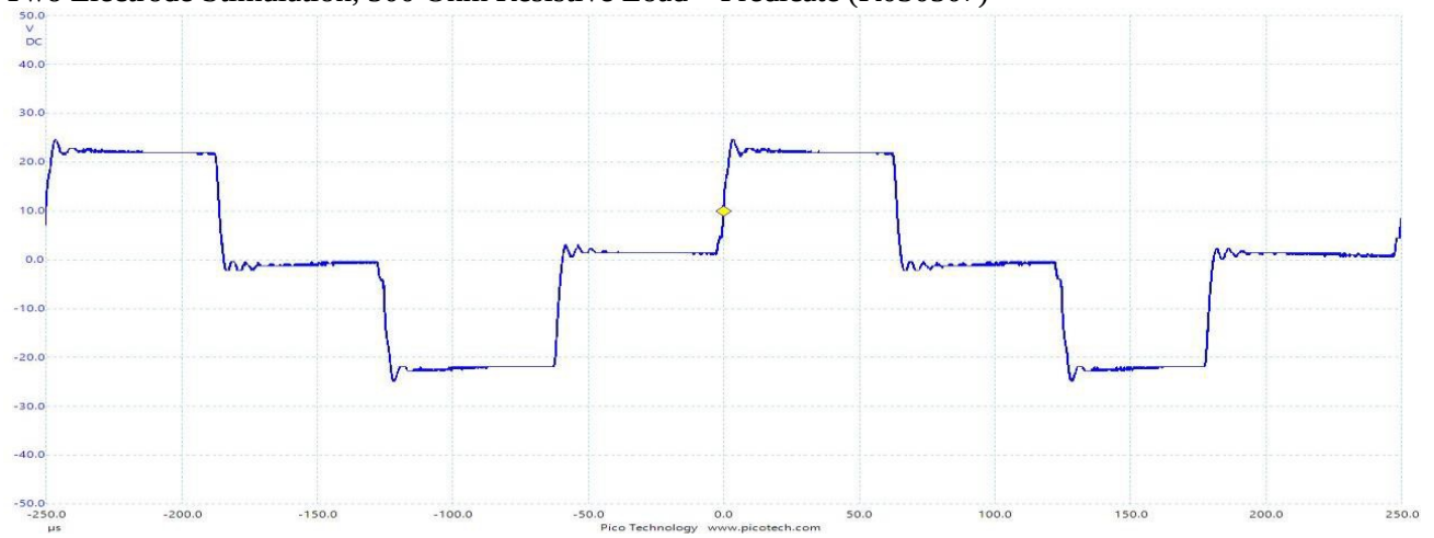
Two Electrode Stimulation, 500 Ohm Resistive Load – Predicate (K030507)
