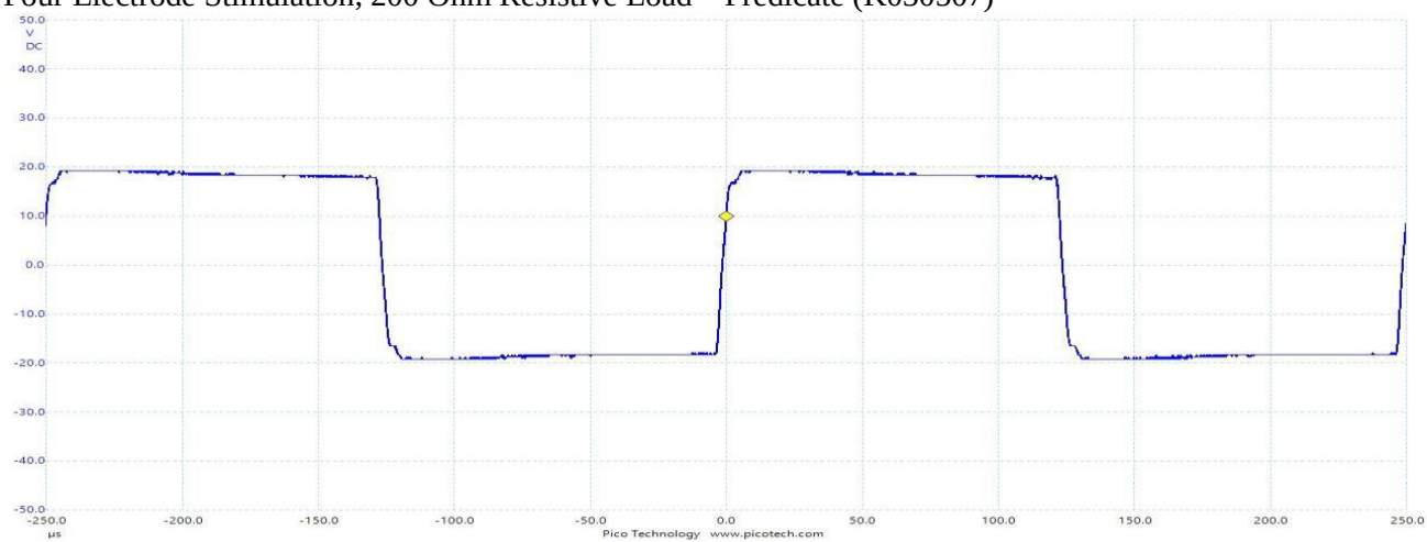
Four Electrode Stimulation, 200 Ohm Resistive Load – Predicate (K030507)
