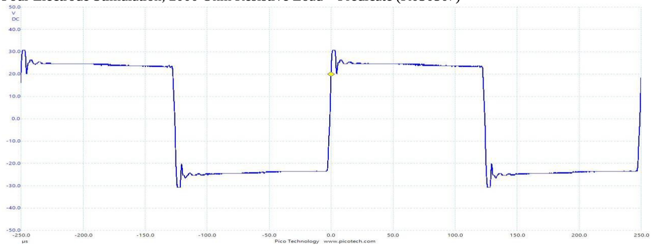
Four Electrode Stimulation, 2000 Ohm Resistive Load – Predicate (K030507)
