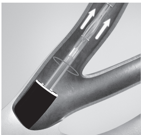
Figure 7a: Advance catheter yellow valve line beyond target location.
