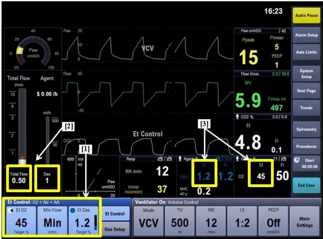
*Figure 1 Aisys CS2 Screen Display (User Interface) with Et Control Activated*
