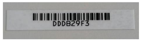
The rating plate is glued on the back of the device housing of the Docking Station. The barcode 128 with the HW-ID (individual hardware identification of the circuit board) is affixed by the manufacturer (EKM) on the rating plate in the field next to the symbol for the serial number on the rear of the device housing. The algorithms and the above representation of the SN are described in the Labelling specification.
