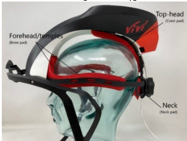
Picture 4: Position and contact areas of foam pads
