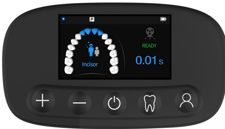
Figure 4. Control panel and the display of the subject device; exposure time is pre-set depending on patient size, tooth group, and image receptor type. The exposure time can be adjusted by pressing the +/- buttons.
