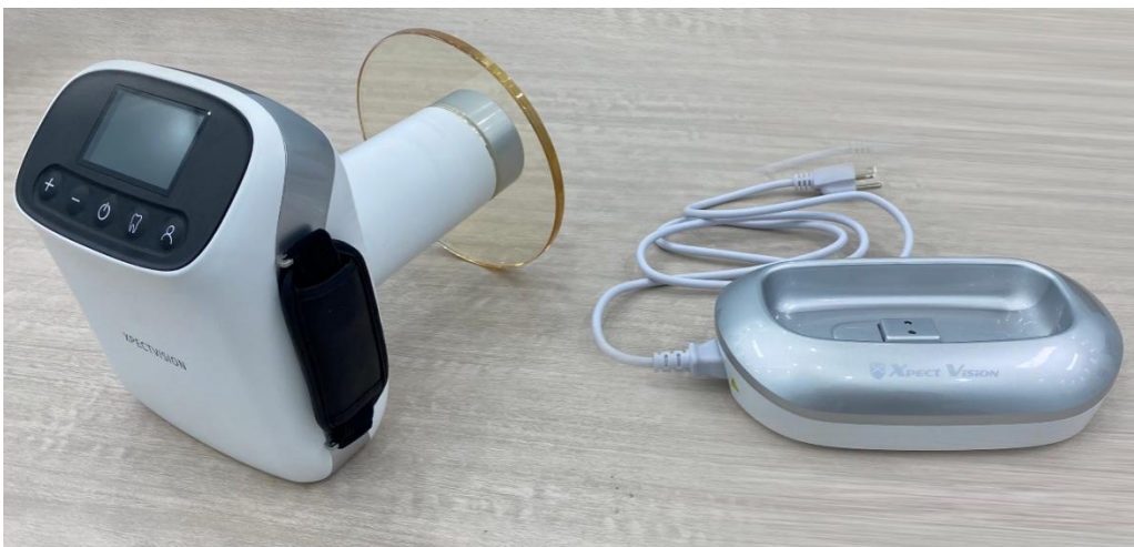
Figure 2. The left is photo of main body and beam-limiting cone of the device; and the right is the photo of charger.
