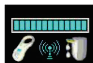
Figure 2-8: Good quality of radio communication to the alfapump ®
