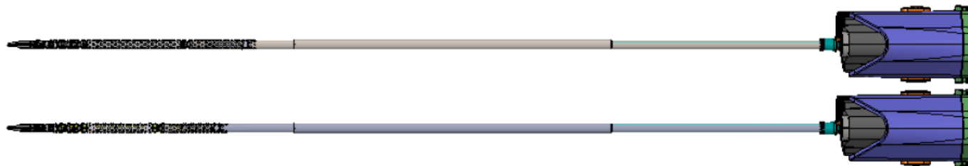
Figure 3: Standard Joggle versus Long Joggle Instrument Comparison – Same Overall Instrument Length
