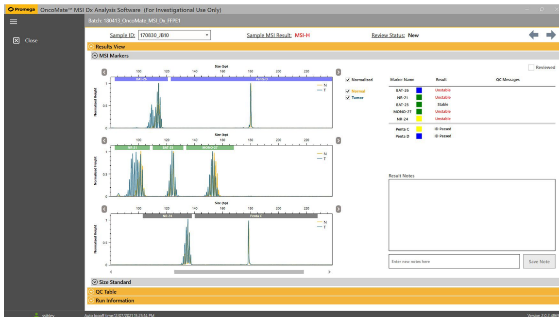
Figure 16. The Sample Data screen. This screen contains sample and size standard electropherograms, marker stability and sample MSI results, the "Reviewed" check box and sample review status, an expandable QC Table section listing QC failures (when applicable), an expandable Run Information section describing the instrument and consumables used for capillary electrophoresis, and a text box for adding user comments.
